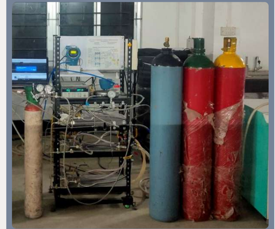
Hydrogen storage and purification system
