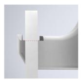
Push the Safe-Lock clamping device so that the mounting of the grinding bowl holder sits centrally in the U-shaped cut-out of the longer projection.
