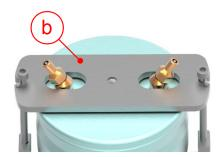
Position the pressure plate (b) with the rubber disk on the bowl as shown in the picture.
