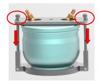
Then tighten both socket-head screws (d) shown in the diagram equally with a hex key and thereby clamp the pressure plate tightly. Ensure that the pressure plate is lying evenly on the bowl lid.
