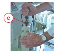
Pre-tension the setting screw (e) manually, then place the provided torque spanner on the setting screw (e) and turn until it clicks. (2.6 Nm)
