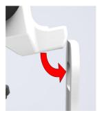
**3.** Hang the short projection of the Safe-Lock clamping device into the other side.
