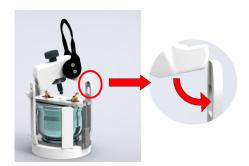
**10.** Hang the short projection of the Safe-Lock clamping device into the other side.
