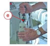
Pre-tension the setting screw (e) manually, and screw it tight using the provided torque spanner. Place the torque spanner provided on the setting screw (b) and turn until it clicks. (2.6 Nm)
