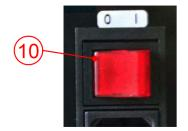
Switch on the device with the main switch (10) on the back side of the device, and release the STOP button.
