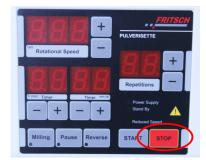
When the device has been switched off, press and hold the STOP button on the front control panel.
