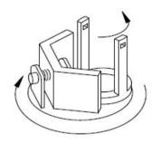
The grinding stock is crushed and ground by grinding balls in a grinding bowl. The centrifugal forces resulting from the rotation of the grinding bowls around their own axes and from the rotating support disc (14) influence the contents of the grinding bowl consisting of grinding stock and grinding balls.
