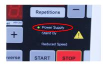
If POWER SUPPLY is flashing, the device is in setup mode. If POWER SUPPLY is not flashing, repeat the procedure.
