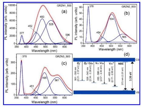
Figure 7. PL spectra of graphene—ZnO hybrid systems after post-growth annealing at 500 °C: (a) NRs (GRZN1\_500), (b) NWs (GRZN2\_500), and (c) NRBs (GRZN3\_500) hybrids. Gaussian fitted peaks are shown with solid lines with peak centers in units of nanometers. (d) Schematic of the band gap defect states tentatively assigned to various PL bands.
