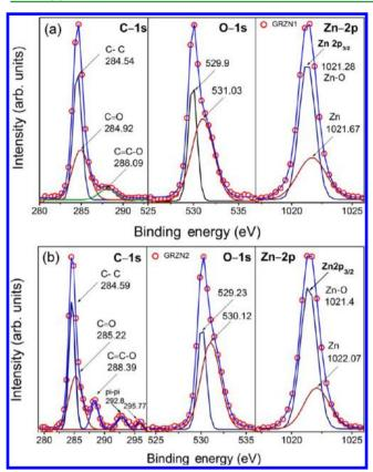
**Figure 8.** C 1s, O 1s, and Zn 2p core level XPS spectra of various graphene—ZnO nanohybrids: (a) NRs (GRZN1) and (b) NWs (GRZN2) showing the graphene sp<sup>2</sup> C, O, and Zn related peaks with fitted spectra as solid lines and symbols as experimental data. Constituent peaks are marked with binding energy values in units of electronvolts.
