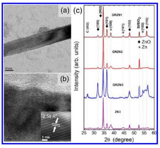
**Figure 5.** (a) TEM images of graphene–ZnO NWs in GRZN2 and (b) corresponding HRTEM image depicting the clear lattice fringe for the ZnO  $\langle 002 \rangle$  plane with its d-spacing shown as an inset. (c) XRD patterns showing *c*-axis orientation of the graphene–ZnO hybrid nanostructures for different substrates.
