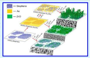
strong UV and visible photoluminescence (PL) from the as-grown and post-growth annealed ZnO NRs, NWs, and NRBs, and the origin of the PL emission is correlated well with the X-ray photoelectron spectroscopy analysis. Our results hint toward an epitaxial growth of aligned ZnO NRs on graphene by a vapor-liquid-solid mechanism and establish the importance of defect engineering in graphene for controlled fabrication of graphene-semiconductor NW hybrids with improved optoelectronic functionalities.
