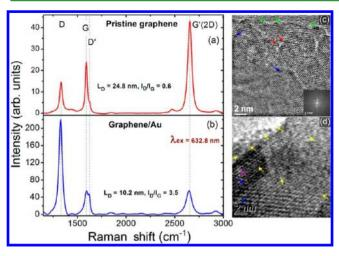
**Figure 9.** Evolution of characteristic Raman modes (D, G, D', and G' bands) of (a) pristine graphene and (b) after Au deposition on graphene. (c, d) Corresponding HRTEM images showing lattice defects. Hexagonal lattice spots of the single crystal graphene are shown in the inset of (c). Color arrows indicate various kinds of defects: green, edge defects; red, line defects; blue, vacancies; and yellow, Au clusters.
