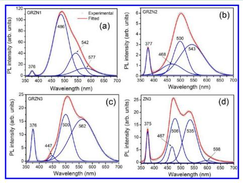
Figure 6. Room-temperature PL spectra of graphene—ZnO hybrid nanostructrues: (a) GRZN1, (b) GRZN2, (c) GRZN3 grown on graphene layer, and (d) ZnO NWs grown without graphene layer (ZN3). Solid blue lines are the Gaussian curves fitted to the experimental data (symbols).
