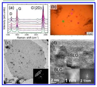
**Figure 1.** (a) Raman fingerprints of as-synthesized graphene transferred to  $\mathrm{Si/SiO_2}$  substrate measured with the excitation wavelength of 514.5 nm and (b) corresponding scanning positions marked in the optical microscope. (c) TEM image of the graphene layer after transferring onto a TEM grid with the corresponding SAED pattern as an inset. (d) HRTEM image of SLG and BLG; inset shows the IFFT and FFT images of the hexagonal lattice spots.
