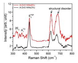
Figure 3. Micro-Raman spectra of the 3% and 6% Al doped ZnO NWs. Characteristic modes are marked with standard notations.
