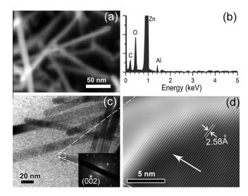
**Figure 1.** (a) FESEM image of the Al doped (6%) as-grown ZnO NWs network with an average diameter 12 nm and (b) the corresponding EDX spectra of the above NWs, confirming the presence of Al in the NWs. (c) TEM image of the above Al:ZnO NWs and the inset shows the corresponding SAED pattern of one of the single NW. (d) High resolution TEM lattice image of the NW taken from one end of the NW.
