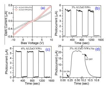
**Figure 4.** (a). Dark current–voltage characteristics of the 3% and 6% Al doped ZnO NWs. (b and c) Reproducible photoresponse behaviors (at 365 nm) of the above two samples. (d) Photoresponse of the 3% Al doped NWs after the surface decoration with Au NPs.
