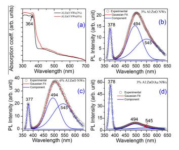
**Figure 5.** (a) UV–Vis absorption spectra of the 3% and 6% Al doped ZnO NWs. Room temperature PL spectra of the (b) 3% and (c) 6% Al doped ZnO NWs. (d) PL spectra of the 3% Al doped NWs after the decoration with Au NPs.
