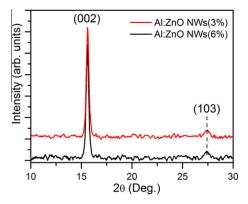
Figure 2. XRD patterns of the 3% and 6% Al doped ZnO NWs, showing the c-axis orientation of the ZnO NWs.
