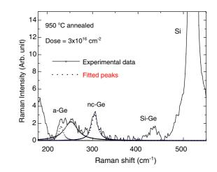
Fig. 2. Optical Raman spectrum of the 950  $^{\circ}$ C annealed sample implanted with Ge ions. Solid line is the experimental data and the broken lines are fitted Lorentzian line shapes. Bonds responsible for the modes are indicated.
