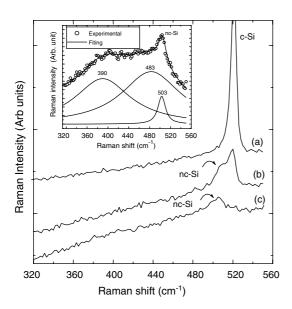
Fig. 3. Optical Raman spectra of the 950 °C annealed samples: (a) Ge1, (b) Ge2 and (c) Ge3. Signature of Si NCs is indicated with arrow for Ge2 and Ge3 samples. The inset shows the background subtracted Ge3 Raman spectrum with constituent peaks fitted to Lorentzian line shapes. Peak positions are denoted by the corresponding wavenumbers.
