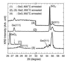
Fig. 1. Grazing incidence X-ray diffraction spectra of Ge implanted and annealed SiO<sub>2</sub>/Si layer. Curve 1: annealing at 800 °C for Ge2, and curves 2, 3: annealing at 950 °C for Ge2, curve 4: annealing at 950 °C for Ge3. Curves 1, 2, and 4 are obtained with grazing angle of  $2^{\circ}$  and curve 3 is obtained with grazing angle of  $3^{\circ}$ .
