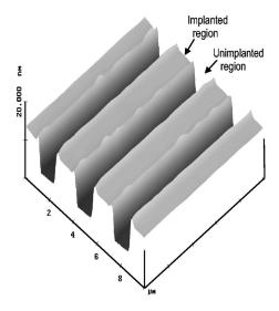
FIG. 1. An AFM image of the swelling observed in 80 keV  $\mathrm{Si}^+$  implanted Si at room temperature, with fluence  $6\times10^{15}$  ions/cm². Unimplanted region corresponds to masked region during implantation.
