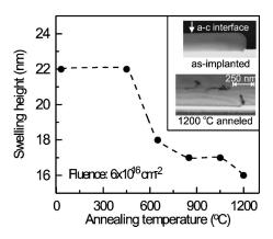
FIG. 2. The saturated step height as a function of post-implantation isochronal annealing at various temperatures, shown for  $6\times10^{16}$  ions/cm<sup>2</sup> implanted sample. Inset shows the XTEM images of the as-implanted and  $1200\,^{\circ}\text{C}$  annealed samples, respectively.
