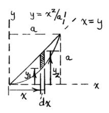
Differential area,  $dA = (y_2 - y_1)dx = \left(x - \frac{x^2}{a}\right)dx$ Rectangle moment of inertia w.r.t. x,  $I_x = \int_0^a \frac{1}{3}y_2^3 dx - \int_0^a \frac{1}{3}y_1^3 dx = \frac{1}{3}\int_0^a \left(x^3 - \frac{x^6}{a^3}\right)dx$
