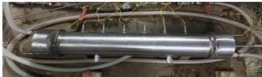
Hydrogen purification system with 40 kg LaNi 4.7 Al 0.3 for storing and purifying ~ 7000 lit. of H 2 . Successfully tested at NTPC Ltd. with 99.99% pure H 2 .
