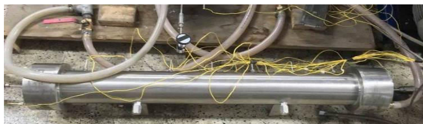
Hydrogen storage reactor g tested with 40 kg MmNi 4.7 Fe 0.3 for fuel cell of 5 kW capacity
