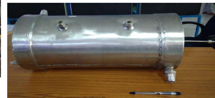
MH based hydrogen storage and cooling system of 10 kW
